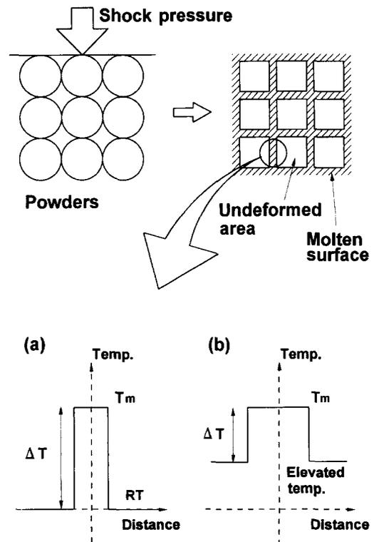
Fig. 5. Schematic illustration for formation of melting layer for room (a) and high-temperature (b) shock consolidation.
