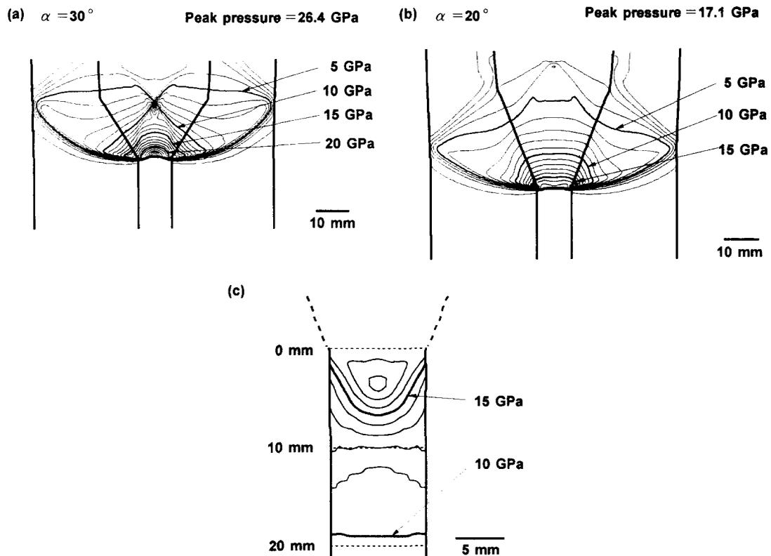
Fig. 3. Calculated water pressure distribution just above powders (converging angle =  $30^\circ$  (a) and =  $20^\circ$  (b)), and maximum pressure distribution in powder part (c).
