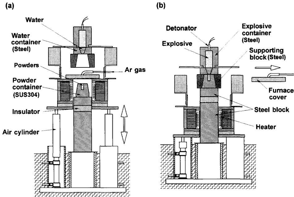
Fig. 1. Set-up for high-temperature shock consolidation.
